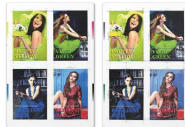
CMYK and RGB+gray(3C) are alternately printed on the margin of the printed sheets. Registration marks are automatically printed on both sides of the sheet to check registration.
